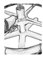
Unlock the foot ring by pushing the top of the inner center hub down.
