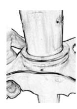
Lock the foot ring in place by pushing on the spokes until the inner center hub extends approximately ½" from the outer center hub.
