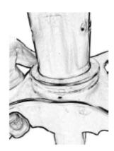
Lock the foot ring in place by pushing on the spokes until the inner center hub extends approximately ½" from the outer center hub.
