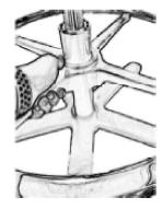
Unlock the foot ring by pushing the top of the inner center hub down.
